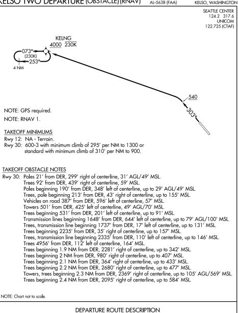
TAKEOFF RUNWAY 30: Climb on heading 303° to 540, then climbing left turn to 4000 direct KELNG and hold. Do not exceed 230K when continuing climb in hold to 4000 before proceeding on course.
