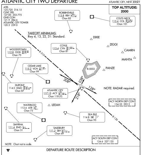
TAKEOFF RWY 4: Climb heading 038° or as assigned by ATC, thence.... TAKEOFF RWY 13: Climb heading 128° or as assigned by ATC, thence....
